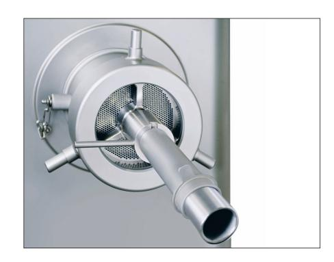
The ULTRA MONO grinders can be equipped with a separator system with lateral outlet and self-regulating spring from cutting set D114 on. The separator systems central and lateral can also be combined. The "Duo Separt" consists of two separating devices which work independent of each other. Thus the separating process can be optimized.
